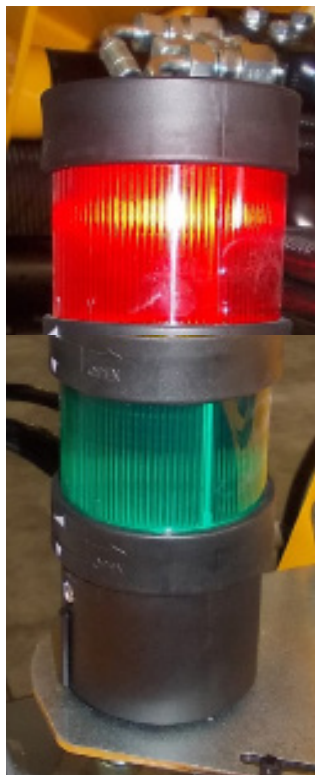
SEMAPHORE. INDICATES STATUS OF MOMENT LIMITER AND LIFTED LOAD - GREEN (OK) - RED (OVERLOAD)
