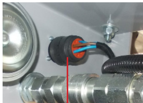
ELECTRICAL CONNECTION POWER PACK
